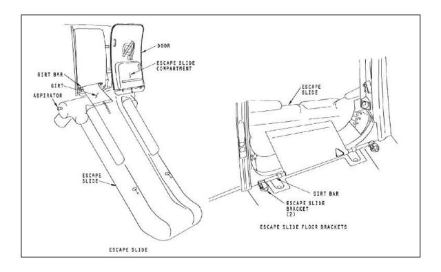
Figure 3. Escape Slide Deployment
