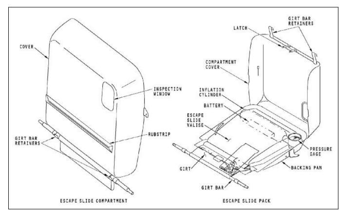
Figure 2. Escape Slide Pack Illustrates the escape slide compartment, and the escape slide pack that it contains.
