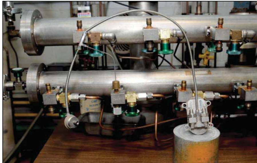
Photo No. 7: pressurizing the P_{T_2}/T_{T_2} sensor to determine leak rate
