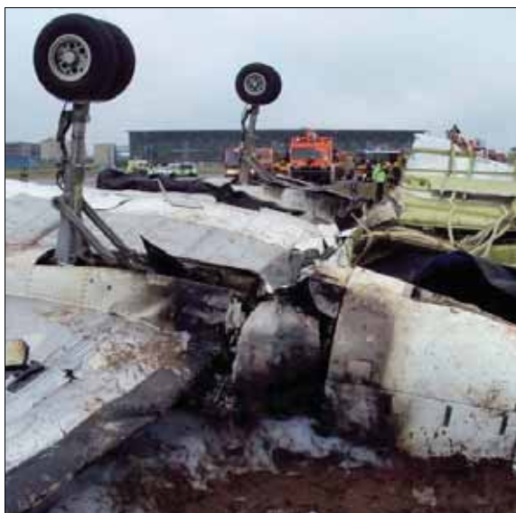
Photo No. 9: Left Engine Fire damage
