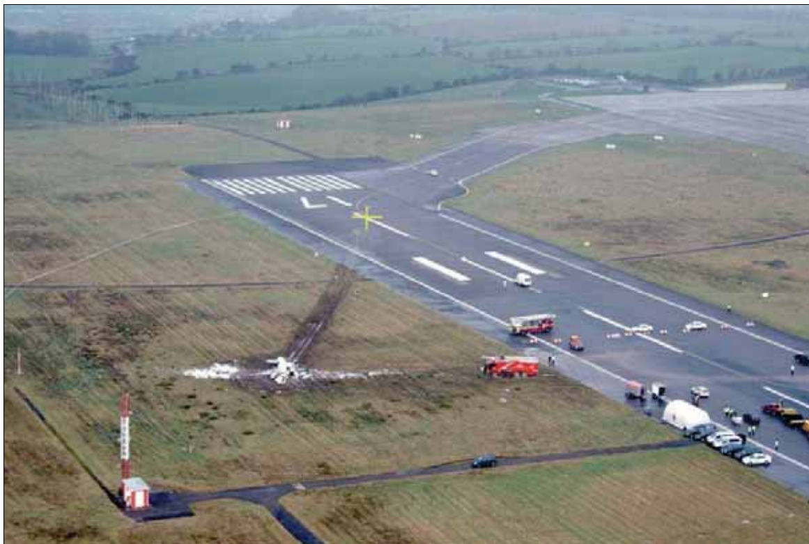
Photo No. 5: Point of initial wingtip contact (identified by the yellow reference mark), debris trail and final position of wreckage
