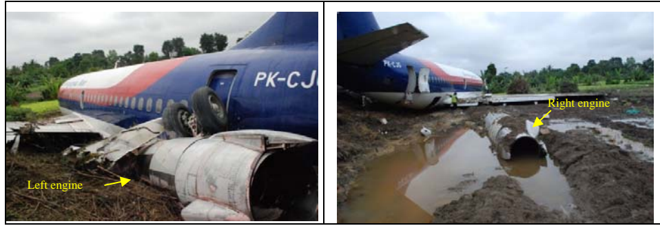
Figure 3: Showing both engines detached
