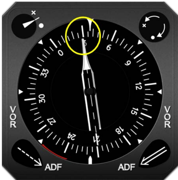
Figure 12. 1625:07: Exemplar of first officer (FO) radio-magnetic indicator (RMI) (no. 2 compass), showing expected true indications with no heading error
