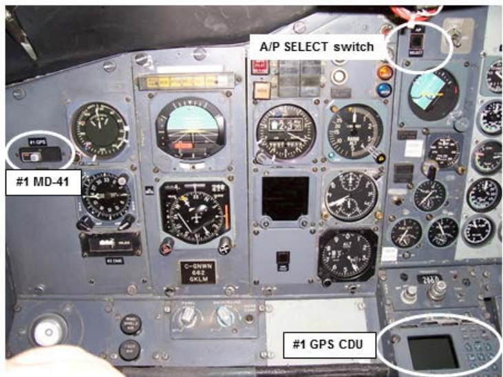
Photo 3. The no. 1 global positioning system (GPS) CDU, no. 1 MD-41 annunciator panel, and A/P SELECT switch
