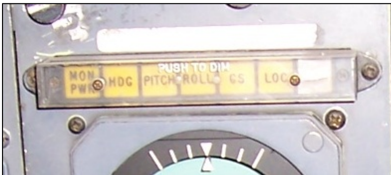
Photo 6. C-GNWN captain's instrument comparator
