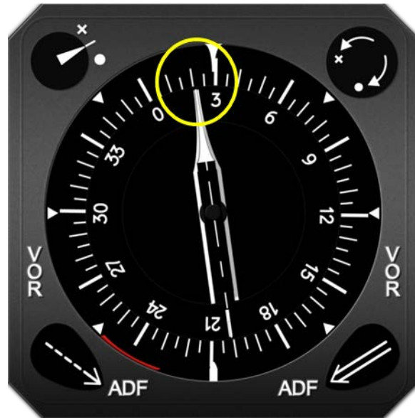
Figure 13. 1625:07: FO RMI (no. 2 compass) showing presumed indications with -8^\circ heading error
