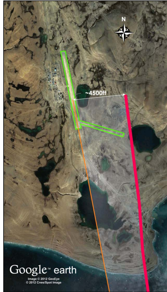
Figure 19. Final approach track relative to runway (image: Google Earth, with annotations by TSB)
