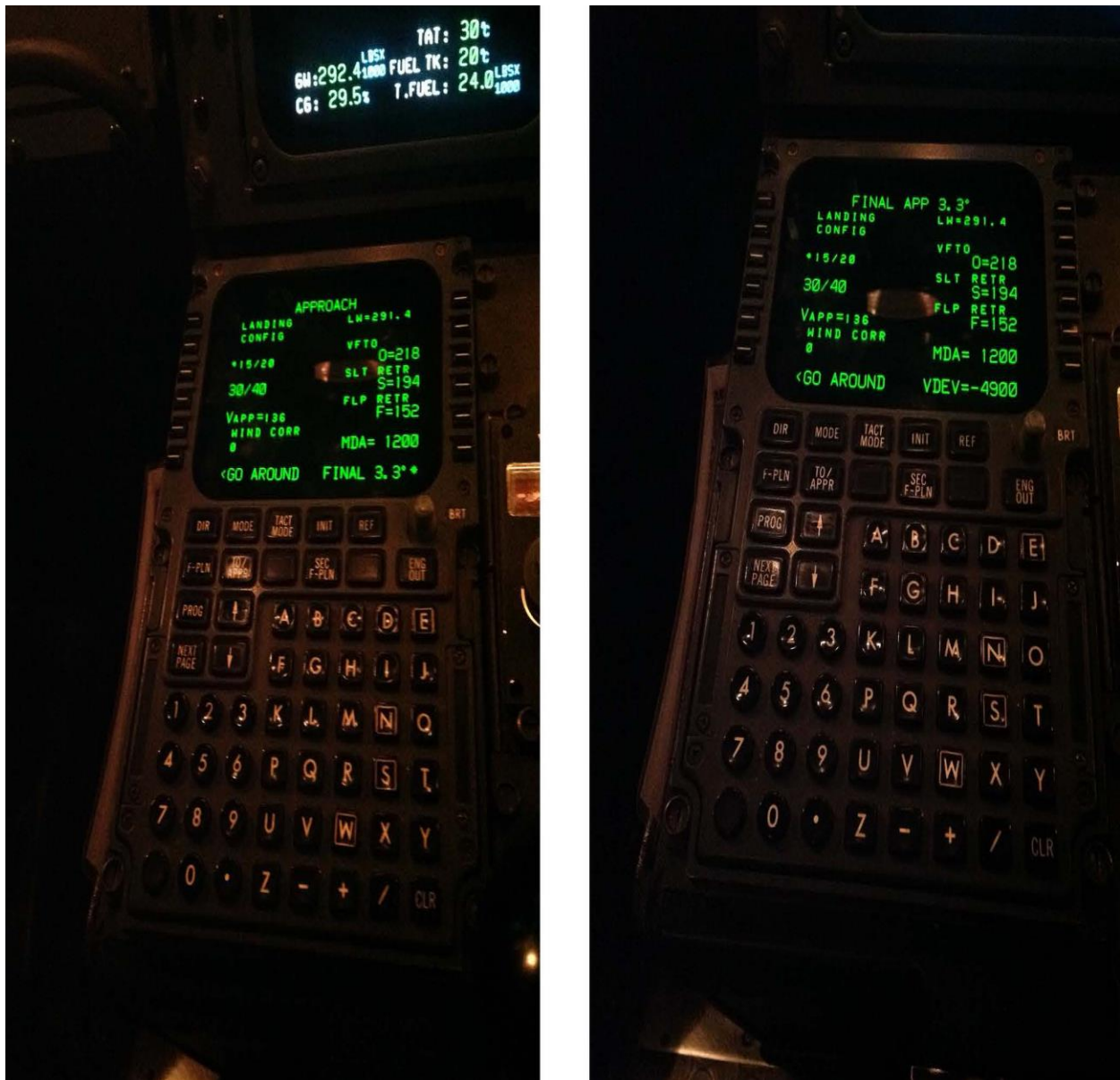
Figure 11. Photographs of an A300 CDU before and after activating final approach mode.
